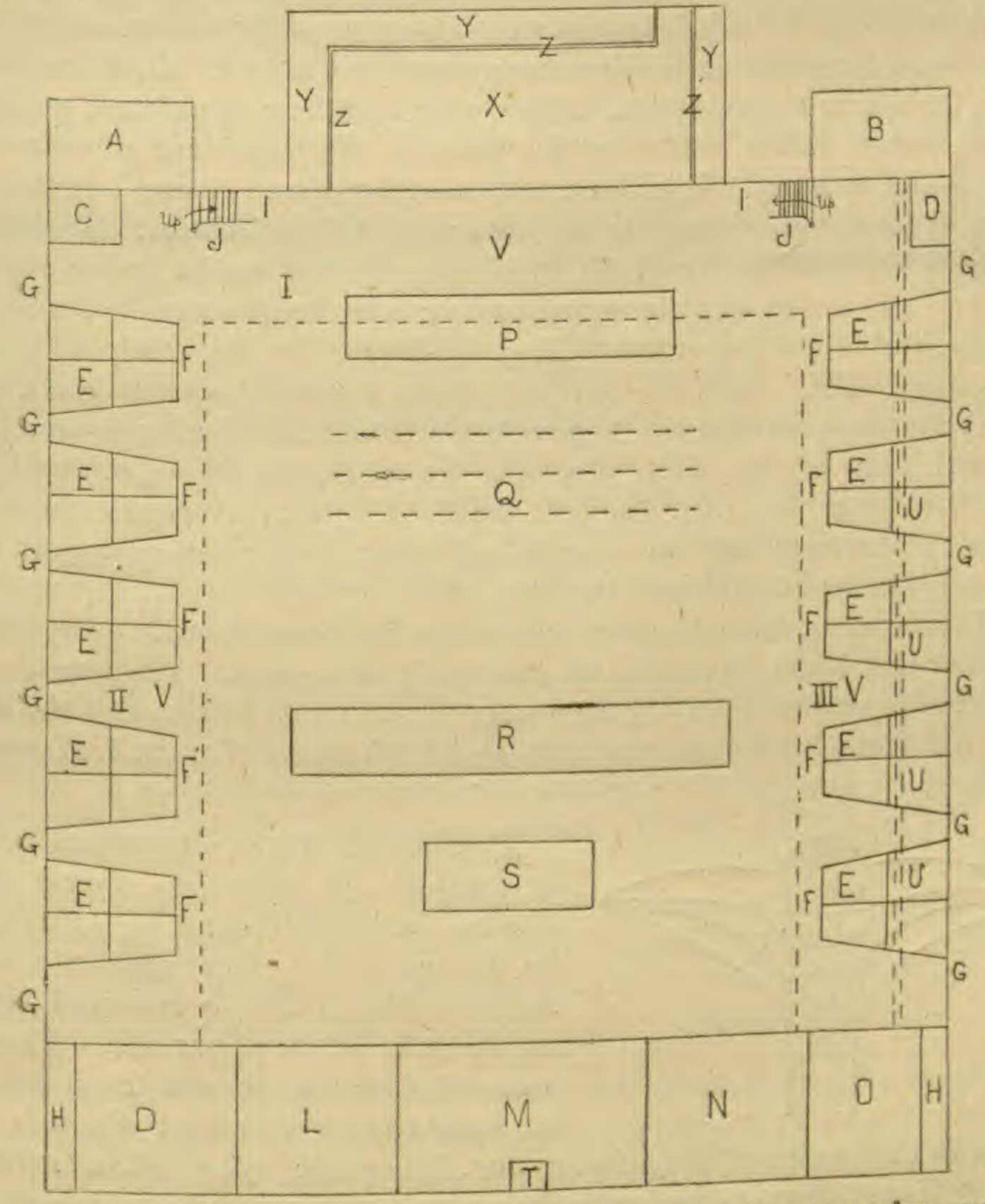
A, teacher's private laboratory. B, small laboratory for special work. C, large spectroscope. D, balances; shelves above hold measuring dishes. E, students' working desks (Bot. Gaz., July, 1885); above each set are spaces for charts and pictures. At F, end of each set of four desks, is a writing-desk and book-shelf. G, windows; brackets are to be
